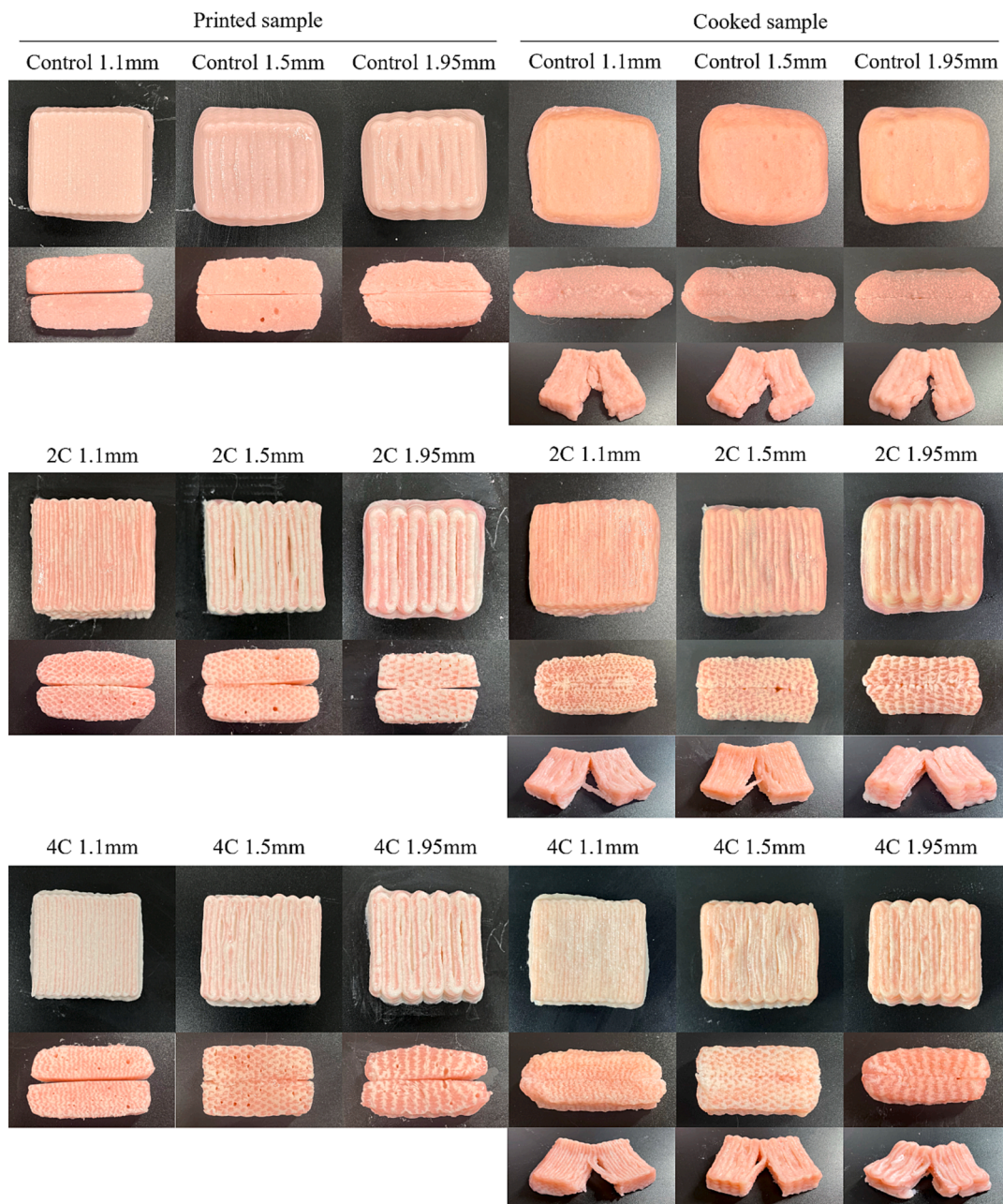
Fig. 6. The images of 3D printed and post-processed cuboid samples with various columns and nozzle diameters. The red coloring was added in PI. (For interpretation of the references to color in this figure legend, the reader is referred to the web version of this article.)
